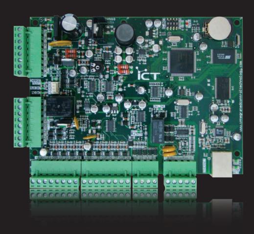
The Protégé® LE Integrated System Controller is the central processing unit responsible for the control of security, access control and automation in the Protégé® integrated system, an advanced technology security product providing seamless and powerful integration of access, security and building automation.
