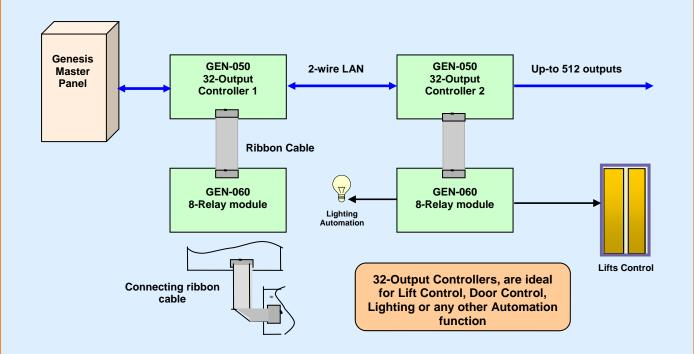
Up to 4 relay modules are supported on the Genesis GEN-050 32-Output controller
